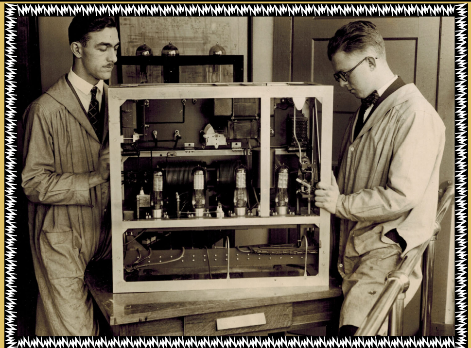
Radio operators C.W. Hancock and C.J. Hartley showing the 64-meter (4.6 MHz) shortwave transmitter designed and manufactured by the A. H. Grebe Company to report on yacht races. The transmitter was installed on Grebe’s personal yacht, the “MU-1,” the name of which was chosen to honor of the “Grebe Synchronphase” broadcast receiver, which made Grebe a wealthy man.
