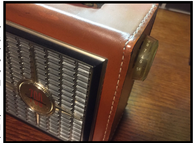
The author's Sears Silvertone transistor radio from 1963 showing the CONELRAD triangle at 640 kHz
