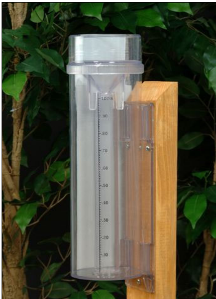
An excellent style manual rain gauge. A reasonable diameter throat improves accuracy. The expanded scale of the internal funnel is readable to 0.01 inch. More than one inch of rain overflows into the outer container. During the winter, the funnel and internal cylinder are removed so that snow can be collected and melted to determine liquid equivalent. (Photo courtesy of Ambient Weather.)
