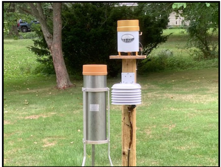
Above: The author’s weather sensors. The standard 8-inch government gauge provides superior accuracy, particularly when measuring the liquid equivalent of snow. It is also used to periodically check calibration of the professional-grade remote-reading tipping-bucket rain gauge. The multiplate radiation shield in the foreground isolates the temperature/humidity sensor from insolation.
