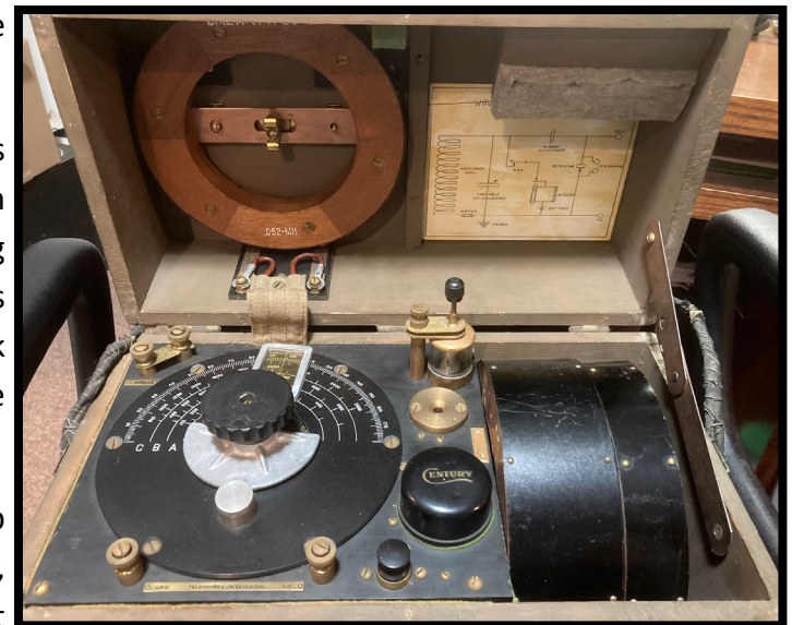
Above: Schematic World War One SCR61 Wavemeter Below: SCR61 from 1918 showing interchangeable coils and calibrated dial
