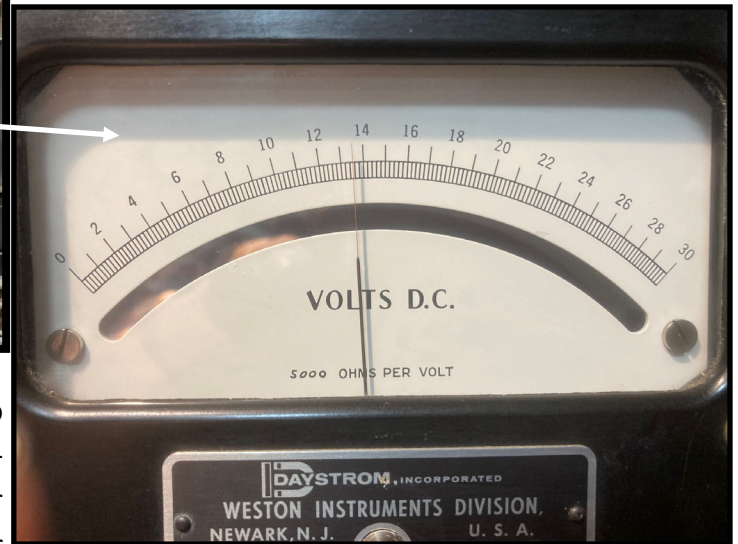
An older lab DC voltmeter used to monitor battery voltage.
