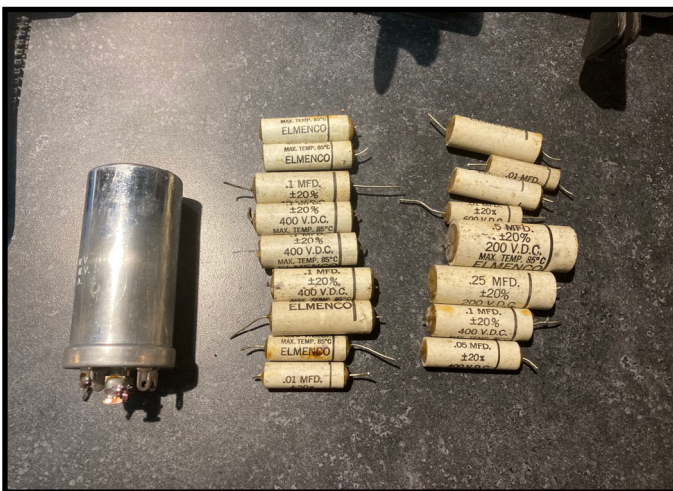
Above: A power supply electrolytic capacitor and some of the paper capacitors replaced.
