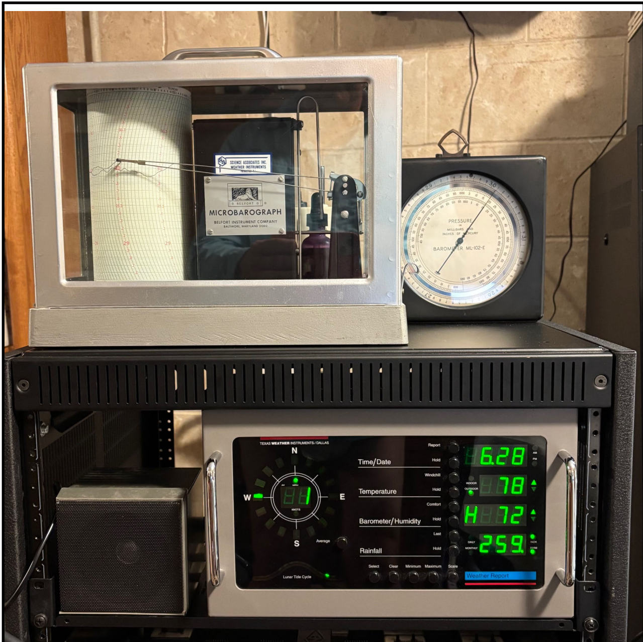
A variety of weather instruments at WB8SIW: On top is a Belfort microbarograph and a military ML-102-E barometer, both extremely accurate instruments. Below is an older “Texas Electronics” weather station purchased for 10-dollars at a local estate sale after the passing of a local TV meteorologist.
