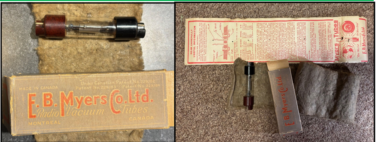
A bit of Canadian Radio History. This Myers Valve was manufactured in Montreal during the early 1920s to avoid patent infringement lawsuits from Deforest, RCA, and others. It was a rugged vacuum tube with a good reputation for performance.
